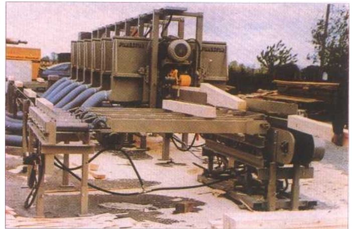
Fig 4. Multi-head thin-kerf machine with feed back system
