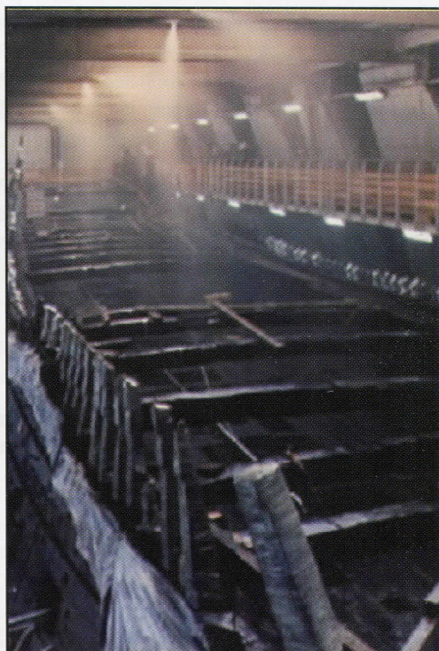
Slika 4: Automatski sistem za prskanje vodenog rastvora PEG-a Figure 4: Automatic system for spraying of water solution of PEG
