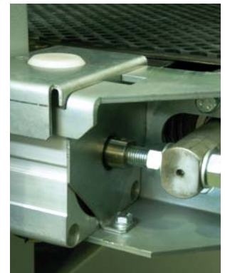
Automatic conveyorbelt tracking
