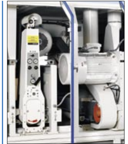
Steel roller with precision bearings followed by a cross sanding unit
