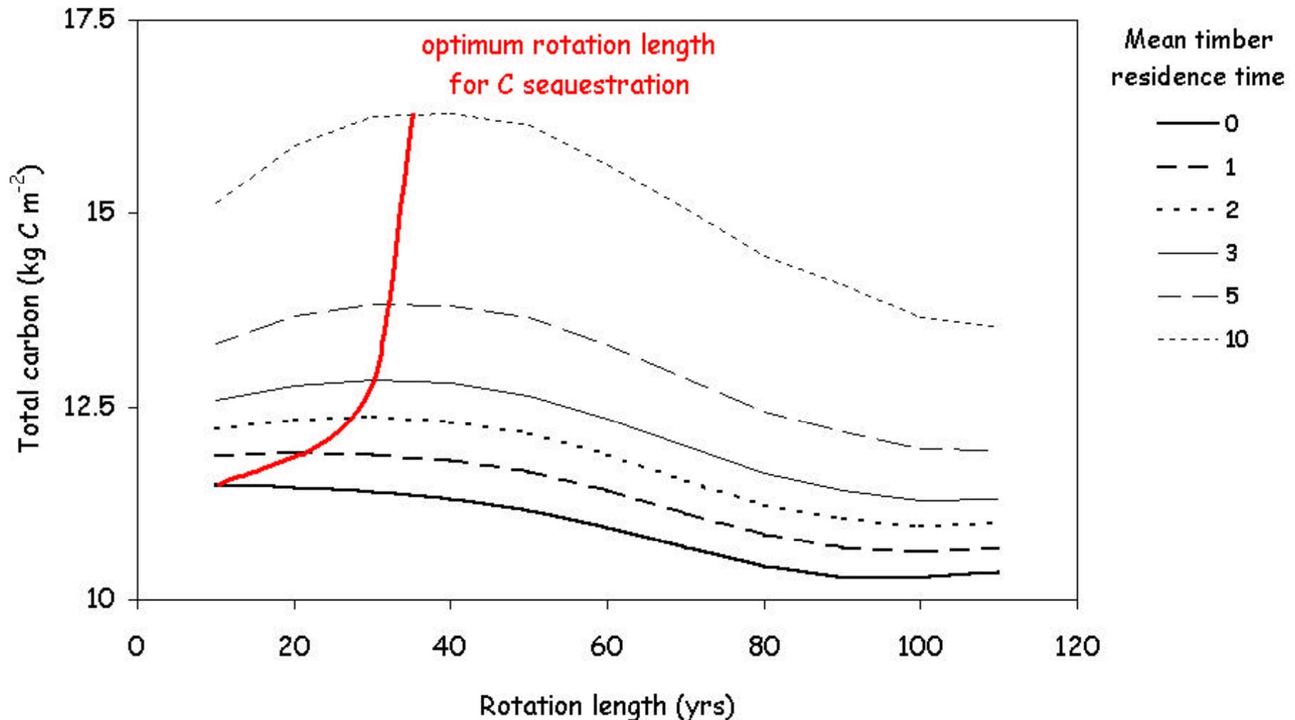
3PG-3 sensitivity analysis. As mean timber residence time in manufactures increases, optimum rotation length is found to increase. Carbon sequestration through changes in timber residence time largely exceed the increase in soil carbon through adaptive management (thick line). Marco Borghetti et al., Università della Basilicata
