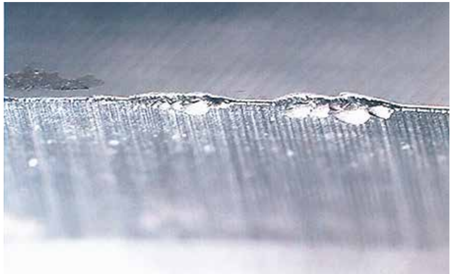
Cutting edge fractures.
