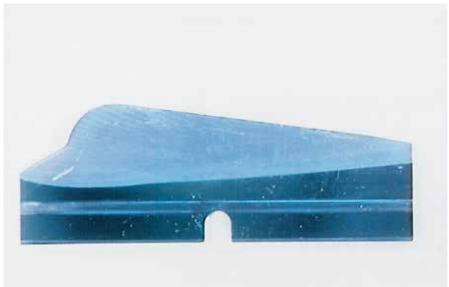
Cutting edge abrasion caused by improper repair
