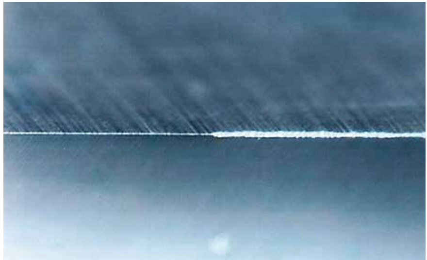
Common rounding of cutting edges after use for spruce
